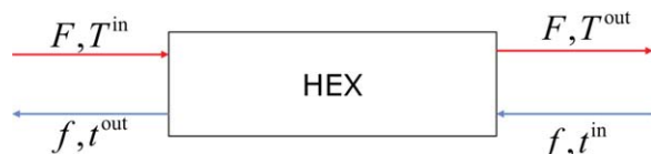
Figure 1. Schematic of a countercurrent two-stream heat exchanger.
